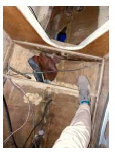
1. the hole under the mainmast bulkhead from where the original keel had broken away (we never found it)
