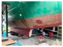
54. and antifouled (note addition of trailing edge fairing piece to reduce drag)
