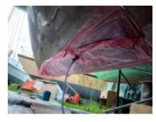
17. a further external stabilising layer pre-keel moulding
