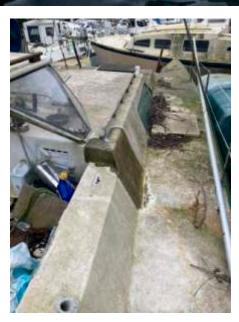
2. starboard side looking forward & a previous repair without UV protection
