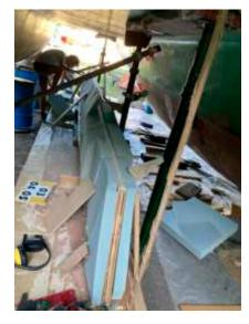
47. Then we glued polyurethane foam sheets and shaped it (surfboard-type construction again
