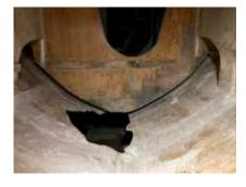
10. mainmast bulkhead cut back and grind prepped
