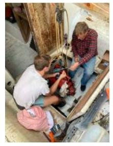
45. A new stern tube, shaft coupling and dripless shaft seal with decent access. Then came what was to be one of the most testing jobs: building a new keel in the summer heatwave. Remember how warm July was?
