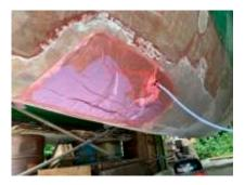
13.1. vacuum bag applied (this photo is actually a pre-bag to check for moisture; the foam core was vac'd after)
