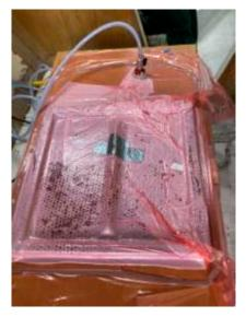
38. Practising vacuum bagging on a hatch lid thanks to Multimarine Composites Ltd for showing me how during work experience back in the day!
